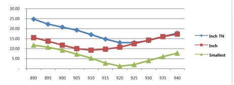
•INCH TN, second tiniest metal tag to NAIL, reads up to 1.0 meters on metal, 30% shorter than INCH (same size, but 1mm thicker than INCH TN). A few of similar size tags from other tag makers reads better, but none is as thin as INCH TN.
