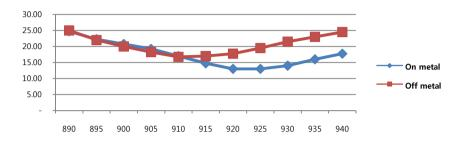
•INCH TN reads shorter by 30% or less off metal (or on non metal surface). It can be applied, therefore, for BOTH metal and off metal application.
