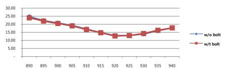
•INCH TN reads same, regardless of whether it is fastened with metal bolt in two holes (located on centers of both ends) or not. Though RF interference is minimal with metal bolts, however, RFcamp recommends not using metal bolts, but 3M 300LSE adhesive or glue for maintaining optimum read performance.
